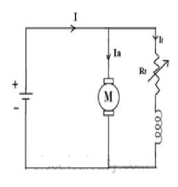
It is seen that **speed of the motor** is inversely proportional to flux. Thus by decreasing flux speed can be increased and vice versa.
